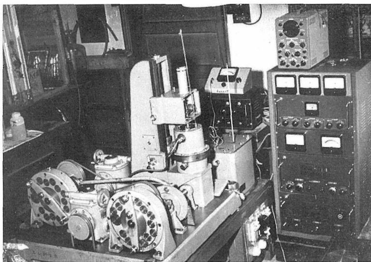
Fig. 1. The view of the parallel disk rheogoniometer. Now it is used as a rotational viscometer. This assembly can be used also for dynamic viscosity measurement.
