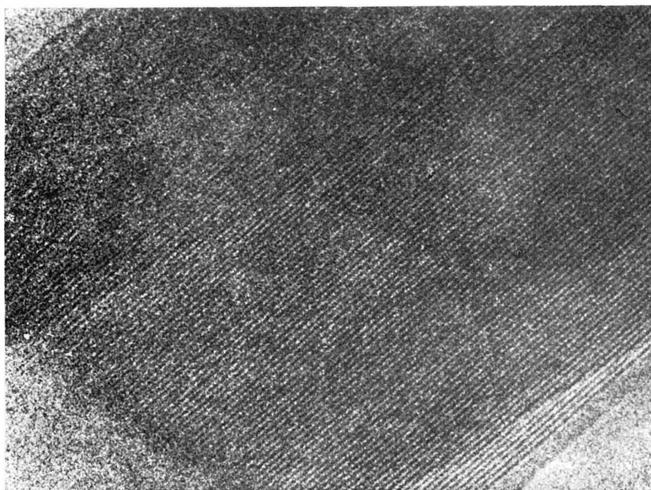
Fig. 7. Lattice image of Cu-phthalocyanine crystal, taken with the 500 kV electron microscope. Accelerating voltage: 500 kV, Lattice spacing: 12.5 \text{ \AA} .
