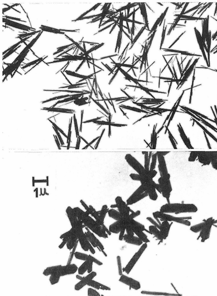
Fig. 1. Electronmicrographs of \alpha -FeOOH, acicular shape of the particles is shown.
