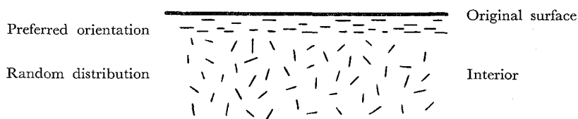
Fig. 11. Arrangement of the hexacelsian in the \text{BaO}\cdot\text{TiO}_2\text{-Al}_2\text{O}_3\text{-SiO}_2 glass-ceramics.
