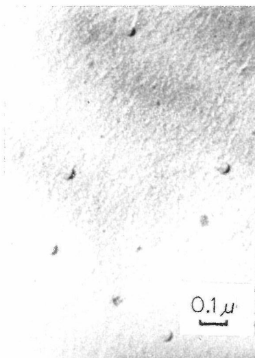
Fig. 1. Electronmicrograph of fractured surface of glass (Ag 0.26, Cl 0.23 wt.%) heated at 600°C for 48 hours after \gamma -ray irradiation.
