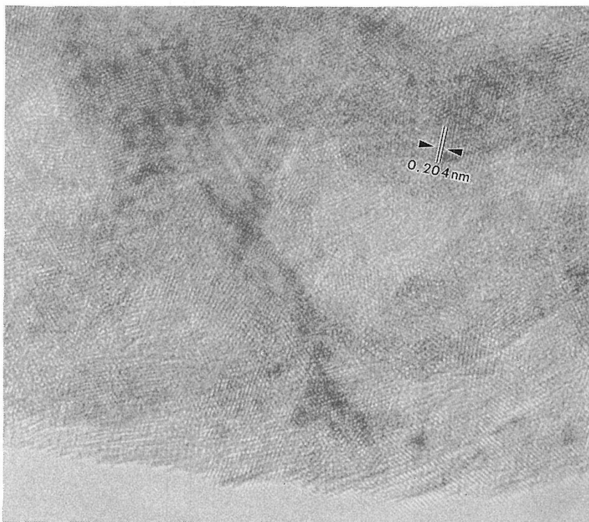
Fig. 5. High resolution electron micrograph of Raney nickel particle developed in 5% NaOH solution.
