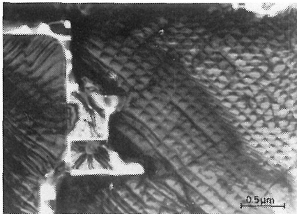
Fig. 9 An electron micrograph of PbTe/SnTe bicrystal, where the substrate SnTe has island structure. Misfit dislocations are observed only at large SnTe islands. Double crosses on smaller islands are extinction contours caused by spherical bending of the island crystals.
