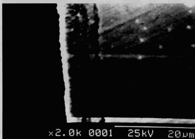
Fig. 3.13. Cross-section SEM image of sample 3 prepared at 0.56 V for 12 h at 723 K.
