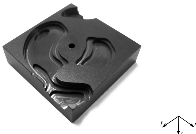
图 5.12 Fabricated dielectric resonator antenna.
