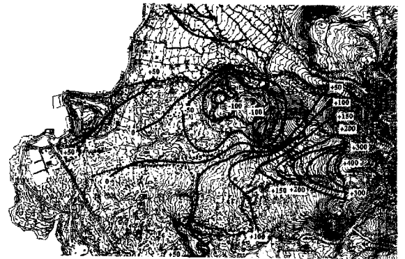
Fig. 5b An equi-potential map in the same area (after topographic correction). (after Hashimoto et. al, 1998)
