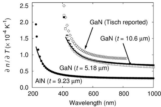
FIG. 3. Thermo-optic coefficients of GaN and AlN compared with reported data from Tisch *et al.* (Ref. 6). Solid lines are polynomial fits of the thermo-optic coefficients of GaN and AlN from Eqs. (2) and (3), respectively.
