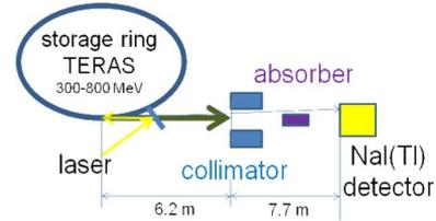
Fig. 2. Schematic drawing of the experimental set-up.
