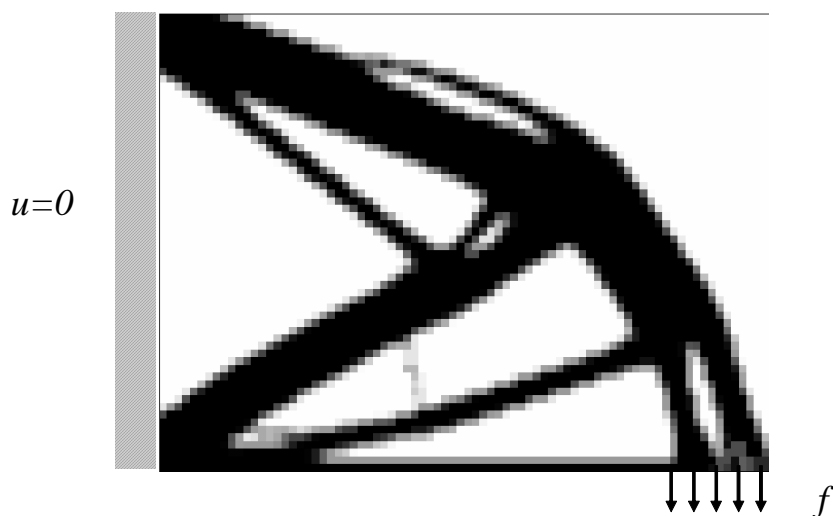
Fig.4.1 Result of cantilever beam optimization.
