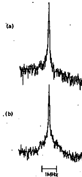
Holes at \Delta = 0 for \theta = 0^\circ (a) and \theta = 10^\circ (b). The broad hole at the bottom of the narrow hole in (b) disappears in (a).
