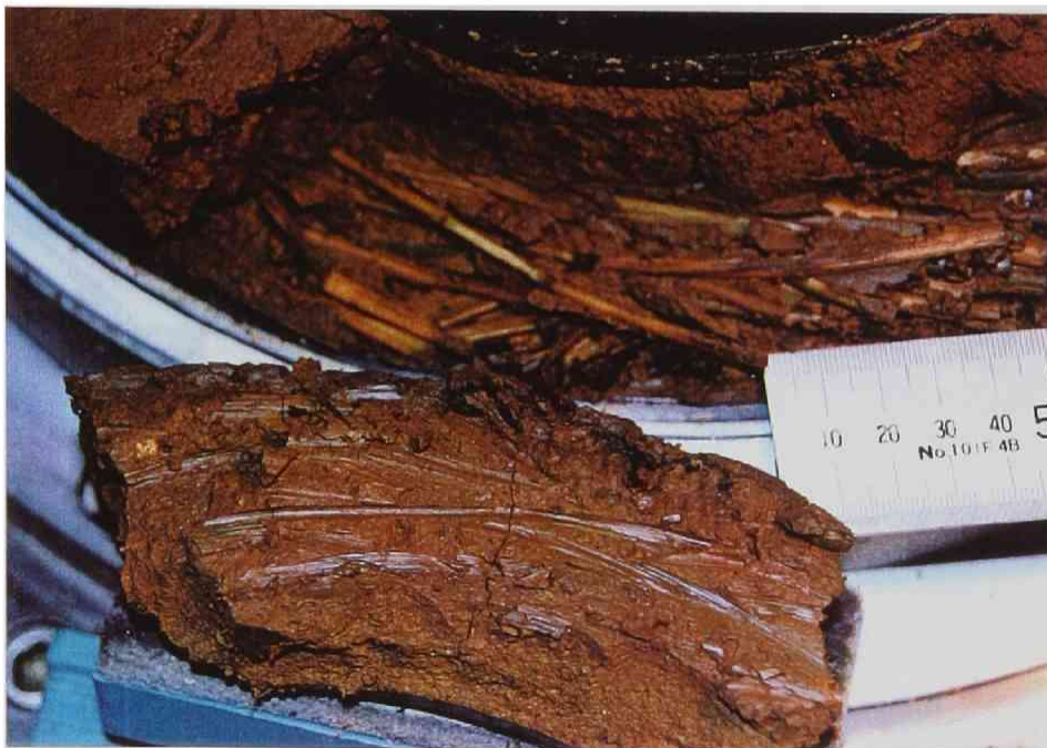
Figure 6.14 Lower part of the shear box after the drained ring-shear test.
