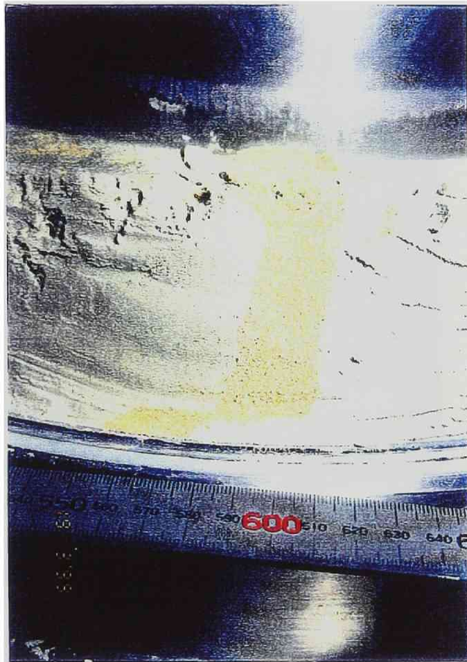
Figure 4.10 Shear deformation of vertically inserted slice of Toyoura sand after 3-cm shear for the complementary test on Test S8r.6 (showing mass liquefaction).
