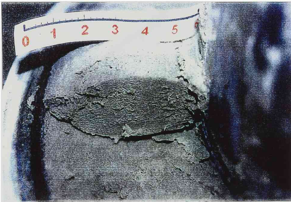
Figure 4.16 Formation of shear zone in the test on dense S8 showing sliding surface liquefaction.
