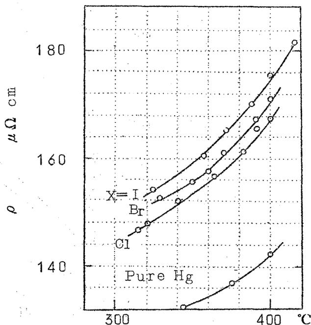
Fig. 1 Resistivity  $\rho$   $\mu$  ohm cm of Hg-1.5 atom % X solutions
