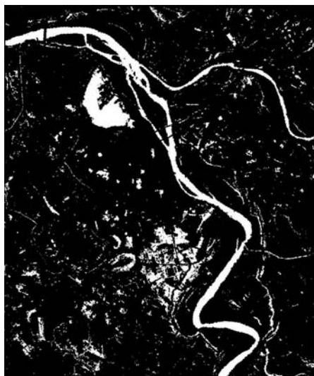
Fig. 3b Water Mask Image Created from Fusion Image on the Left
