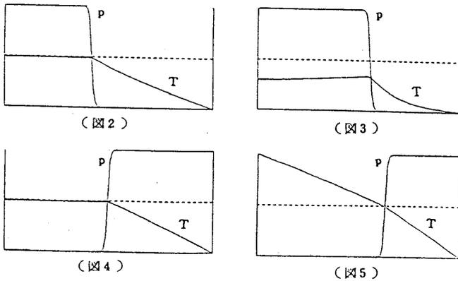
(図2)は undercooling (図3)は hypercooling
