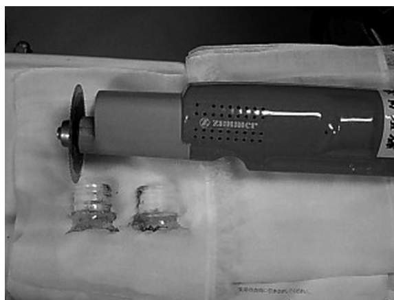
Fig. 2. An electric plaster cutter for an orthopedic surgery that we used and the dual-partitioning PET bottle mouth.
