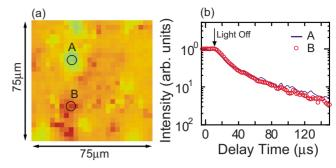
FIG. 6. (Color online) (a) Spatial image of the PL intensity due to  ${}^{5}D_{0}$ - ${}^{7}F_{2}$  transition of the GaN: Eu<sup>3+</sup> epitaxial film under 325 nm light excitation at 10 K. (b) Spatially resolved PL decay profiles monitored at positions A (solid line) and B (open circles) under 325 nm light excitation at 10 K.
