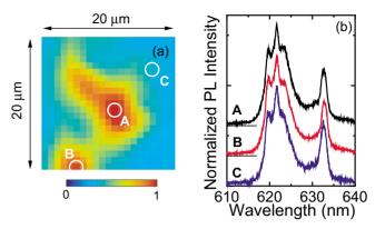
FIG. 4. (Color online) (a) Spatial image of the spectrally integrated  $Eu^{3+}$  PL intensity from 615 to 640 nm under 325 nm light excitation at room temperature. (b) Spatially resolved PL spectra monitored at positions A– C under 325 nm light excitation at room temperature.
