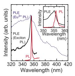
FIG. 2. (Color online) PLE spectra of the Eu<sup>3+</sup> PL monitored at 622 nm (broken line) and of the bound-exciton PL monitored at 400 nm (solid line) at 20 K. The PL spectrum at the highest energy is shown under 325 nm excitation. The PL spectrum under 325 nm excitation and the PLE spectrum monitored at 400 nm are shown in the inset.
