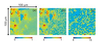
FIG. 7. (Color online) Spatial images of the PL intensity due to (a)  ${}^{5}D_{0}{}^{-7}F_{2}$  and (b)  ${}^{5}D_{0}{}^{-7}F_{1}$  transitions of Eu<sup>3+</sup> ions under 325 nm light excitation at 10 K. (c) Spatial image of the PL intensity ratio of the  ${}^{5}D_{0}{}^{-7}F_{2}$  to  ${}^{5}D_{0}{}^{-7}F_{1}$  transition.
