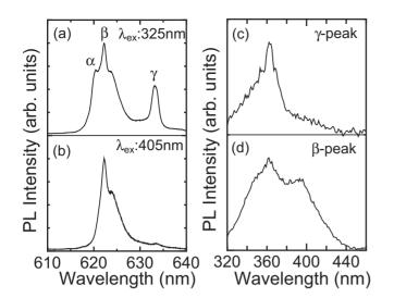
FIG. 3. PL spectra under (a) 325 nm and (b) 405 nm light excitation at room temperature. PLE spectra monitored at PL peak (c)  $\gamma$  and (d)  $\beta$  at room temperature.
