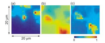
FIG. 5. (Color online) (a) Spatial image of the intensity of the bound-exciton PL monitored in the spectral range from 350 to 360 nm under 325 nm light excitation at 10 K. Spatial images of the PL intensity due to  ${}^{5}D_{0}{}^{-7}F_{2}$  transition of Eu<sup>3+</sup> ions monitored in the spectral range from 615 to 640 nm under (b) 325 and (c) 405 nm light excitation at 10 K.
