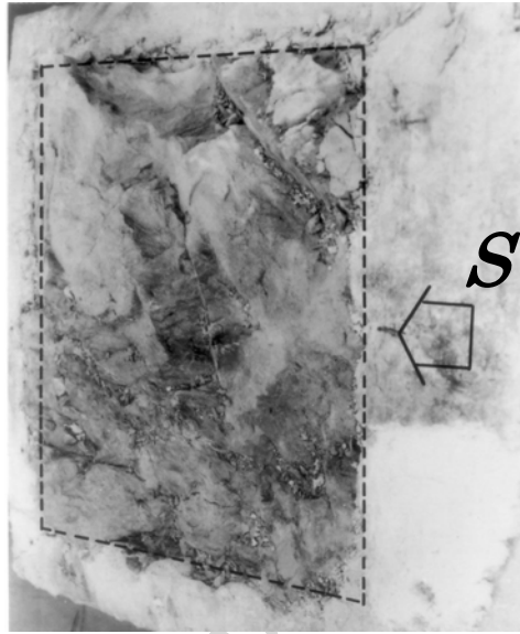
Photo 3 Fractured plane of the test block. This photo was printed by turning over the negative so that the right and the left hand sides along the direction of the shear load appear in the same position as in the other figures.
