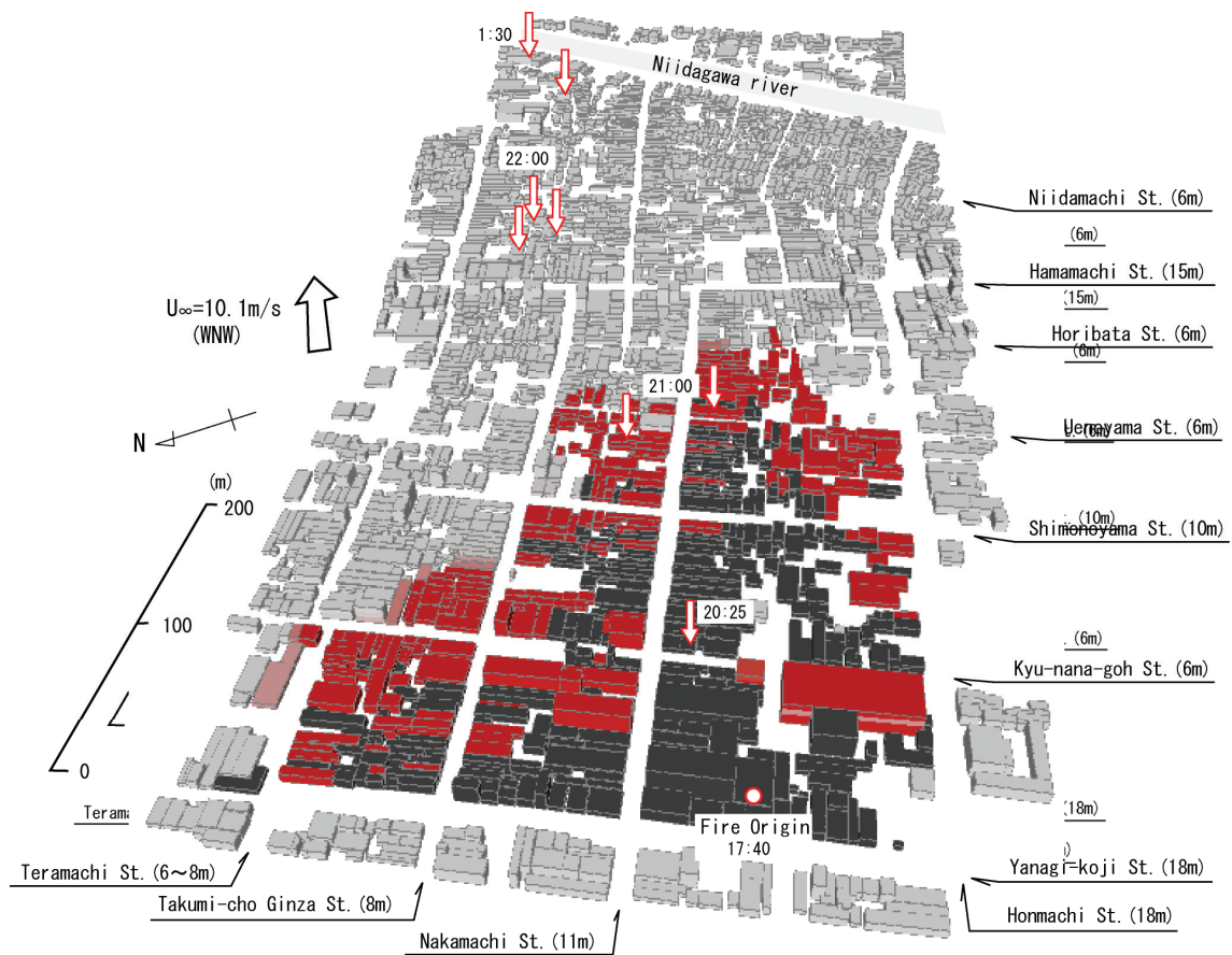
Fig.14. Result of fire spread simulation at 22:00 (4hrs 20min after the outbreak of fire), Oct. 29th. Arrows indicate buildings of secondary fire origin initiated by firebrands.
