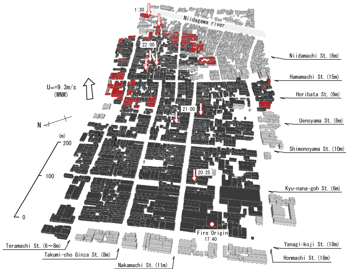
Fig.16. Result of fire spread simulation at 2:00 (8hrs 20min after the outbreak of fire), Oct. 30th. Arrows indicate buildings of secondary fire origin initiated by firebrands.
