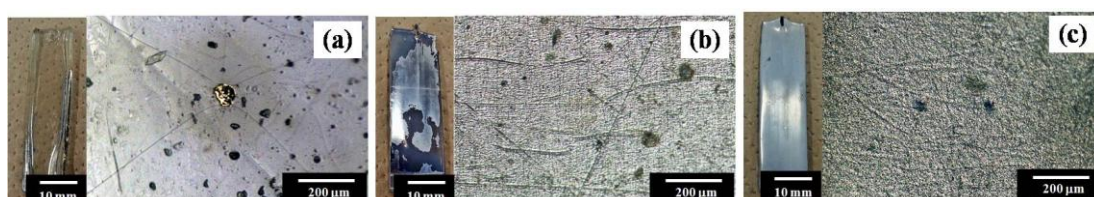
Figure 4.13. Digital camera (left) and optical microscope images (right) of surfaces for (a) Ni-P-plated neat SAN substrate, (b) Ni-P-plated SAN/PEEA blend (95/5) substrate and (c) Ni-P-plated ABS substrate; the polymeric substrates were impregnated with the Pd catalyst by \text{scCO}_2 infusion at a \text{Pd(hfa)}_2 concentration of 9.52 \times 10^{-4} \text{ g-Pd(hfa)}_2/\text{g-CO}_2 .
