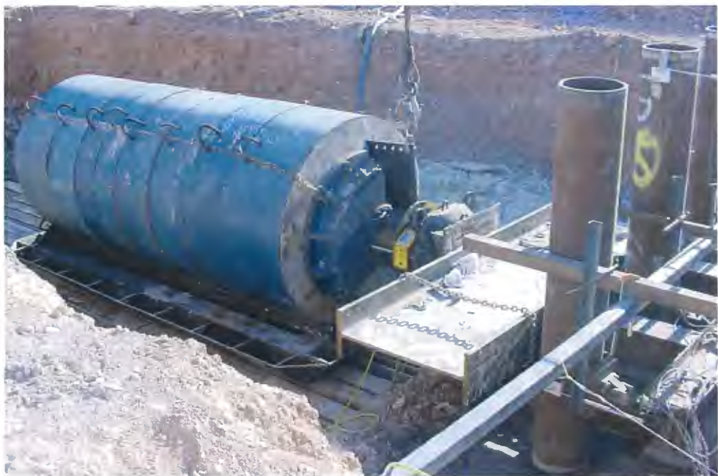
Fig. 4.7 Photograph of the statnamic device used to dynamically load the 15-pile group
