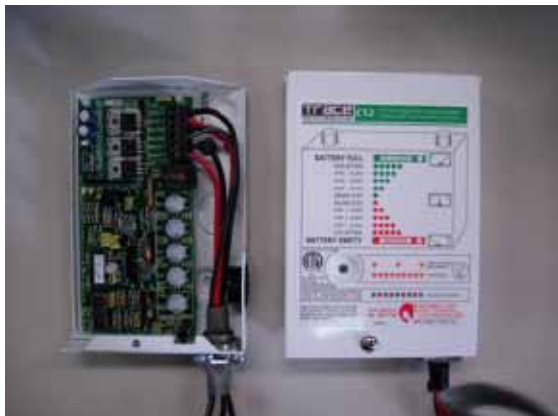
c. Controller of solar panel (C12)
