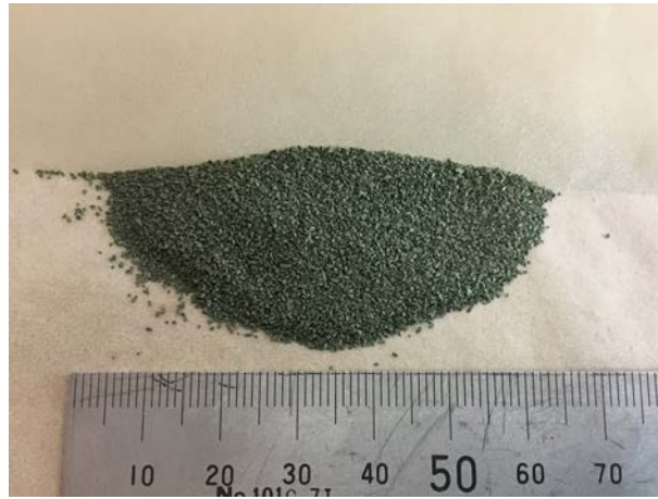
Fig. 3.1 Crushed NiO-YSZ catalyst before the reduction process.
