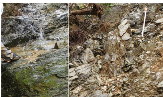
Fig. 8 Non-deformed pelitic schist (left) and gravitationally buckled pelitic schist (right).
