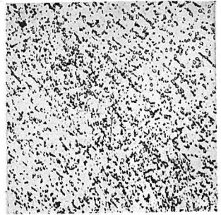
Photo 3. 7.0% Al Quenched from 680°C in ice-water.
