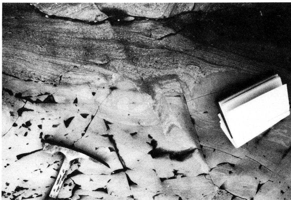
Fig. 12. Thixotropic deformation in the siltstone.
