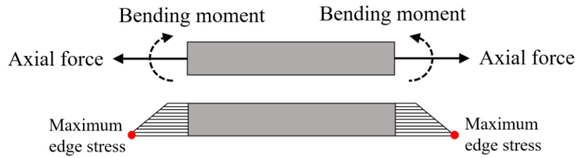
Fig. 4 Illustration of internal force and maximum edge stress of beam element
