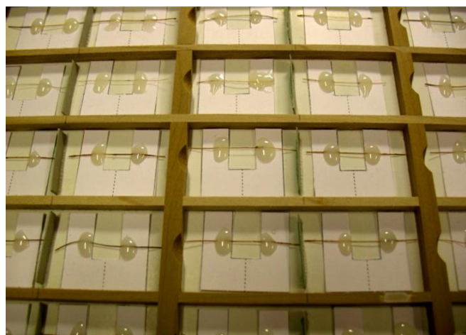
Figure 2.11 Specimens under 60% relative humidity and 20°C condition.
