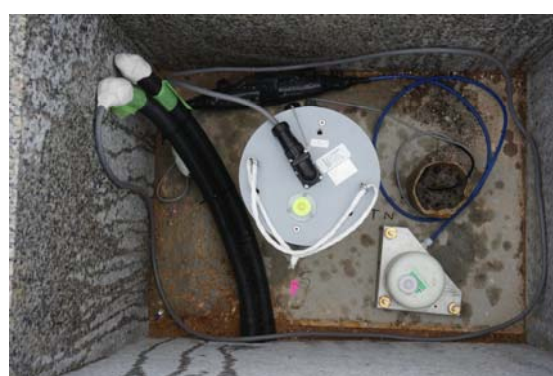
Photo 2: (a) (upper) Newly constructed DP.YKEP (Summit of Yake-dake volcano) station. Main part of the equipment center) and a pillar for the proton precession magnetometer (left behind) are seen. (b) (lower) Instruments installed at DP.YKEP. Short period seismometer, tiltmeter (lower right), and high sensitivity thermometer (upper right) are seen.
