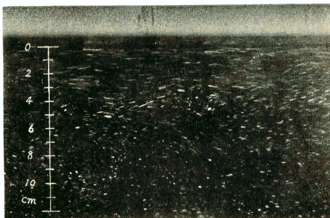
Photo. 3 A steady state of currents, large scale eddies occur
