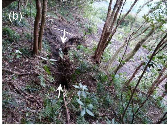
Photo 3 Head of a landslide (a) and a tension crack (between the white arrows) near the landslide scarp (b).
