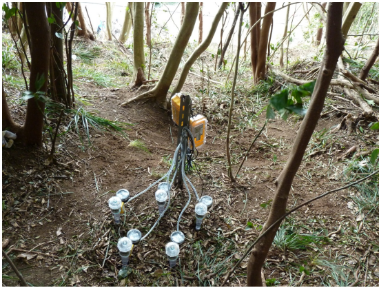
Photo 4 Tensiometers to measure the pressure head in soils at P1 shown as A7 in Fig. 5. Depth of the measurement is 25, 55, 85, 115, and 145 cm.
