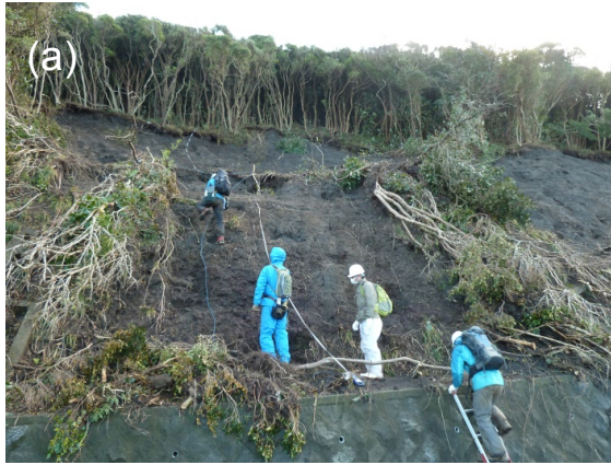
Photo 3 Head of a landslide (a) and a tension crack (between the white arrows) near the landslide scarp (b).
