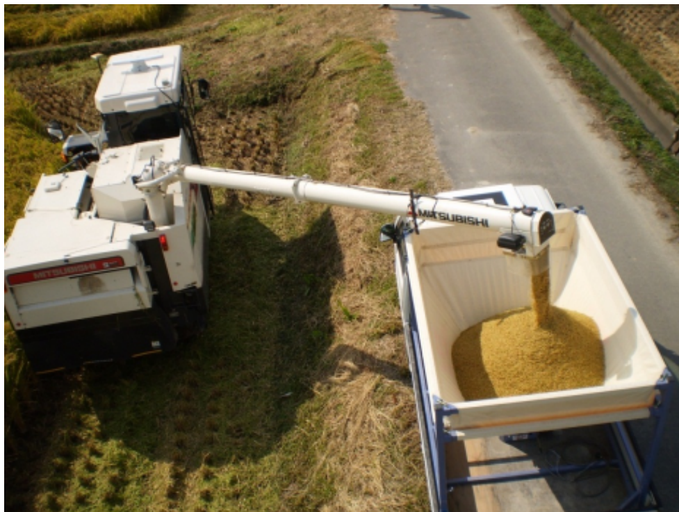
Fig. 4.3. Combine harvester unloading grains into grain container.
