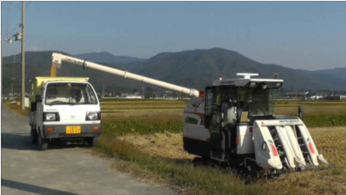
Fig. 5.12. Combine robot unloading grain into grain storage container.
