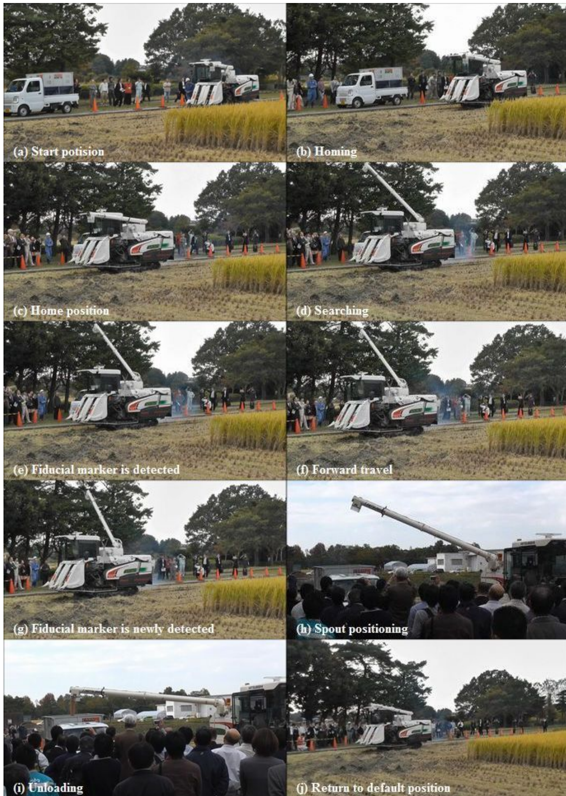
Fig. 5.14. Scenery of autonomous unloading system actually working.
