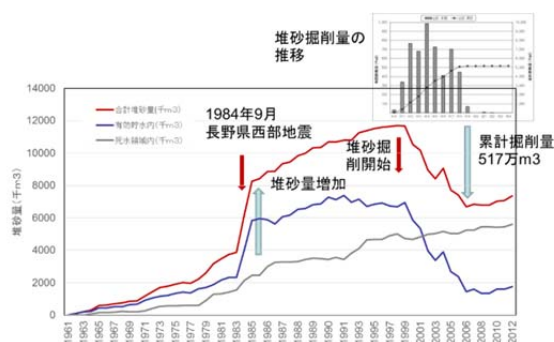
Fig. 4 Change of reservoir sedimentation (in the active storage and the Dead storage) in Makio Dam
