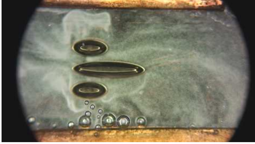
Figure 4.5: (Color online) Micrograph of transient flow around V_{0w} \sim 8 V, when V_0 is increased from 0 to 15 V. Here, V_{0w} = 15 V, f = 50 Hz, w = 1.6 mm, c/w = 0.065 , b_1/c = 4.6 , b_2/c = 2.3 , \delta/w = 0.05 , t_s U_c/w = 0.00405 , and E_0 = 9.4 kV/m.
