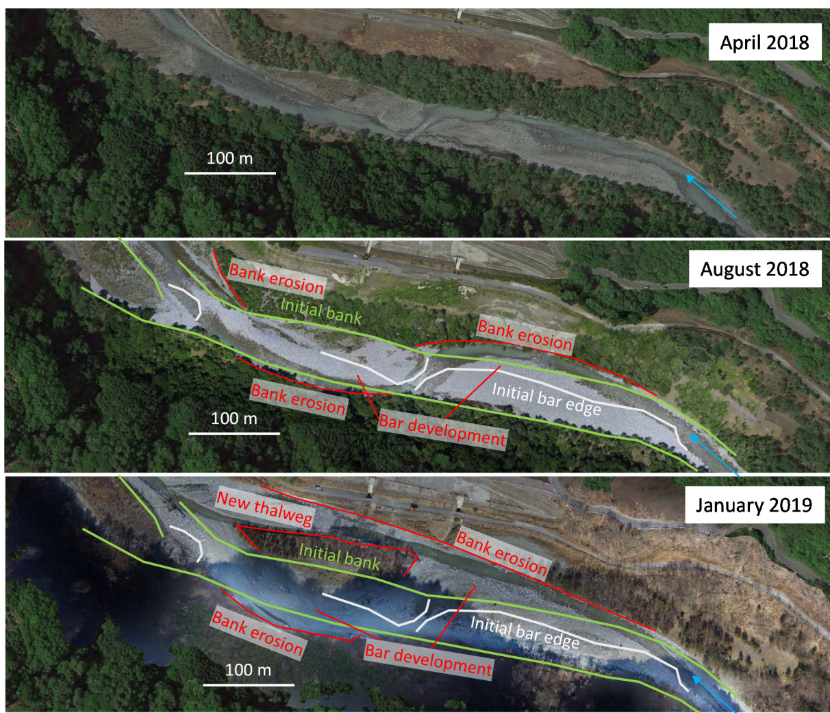
Fig. 10 Channel change (gravel bar development, bank erosion, new thalweg formation) at near 1.6k
