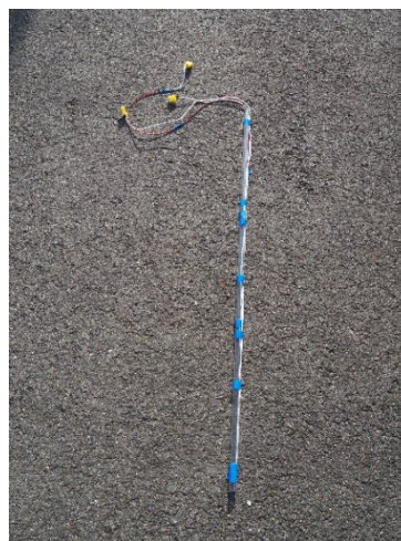
Photo 3 The state of the thermocouples inserted into the PVC pipe.
