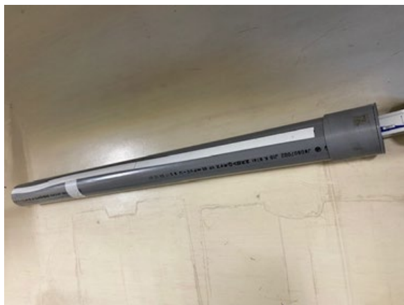
Photo 1 PVC pipe case used as a magnetometer sensor container.
