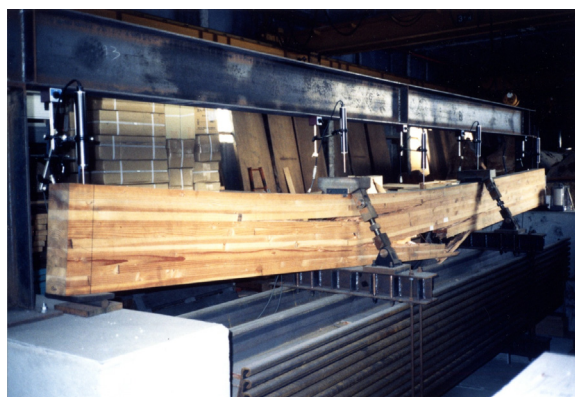
Photo 11 A creep test for the laminated timber
