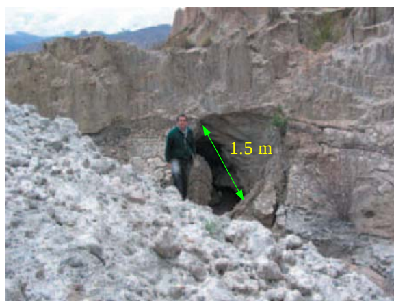
Fig. 1 Natural tunnel through a landslide dam in Allpacoma valley, La Paz, Bolivia, formed due to piping failure (Hermanns, 2005).
