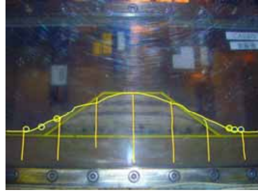
Fig. 5 Measured deformation of embankment on dense foundation ground after shaking (Case6)
