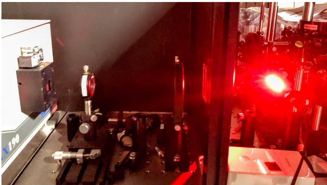
Figure 4.14. Spectral resolution measurement using a neon lamp
