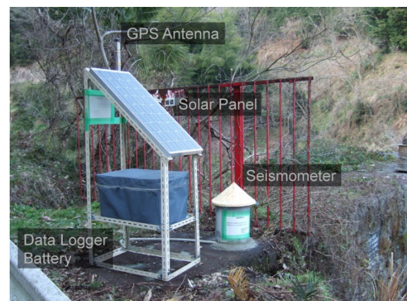
Photo 1 Seismic observation equipment installed at temporary station SL19 along survey line JJ'. The seismometer was installed on top of a sabo dam and covered with a PVC pipe and a jingasa (a conical hat) for protection. The data logger and battery were stored in the box beneath the solar panel.
