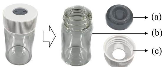
* (a) Fluoride rubber plug, (b) Glass vial, (c) Plastic lid.
