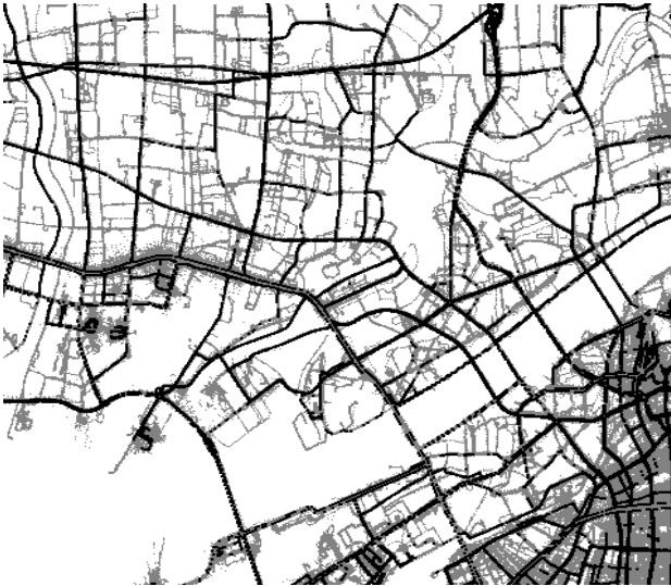
Figure 7 Probe density map: Black lines are high frequency network and gray lines are low frequency network
