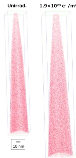
Fig. 2. Atom maps of Re for W-5%Re alloy before and after electron-irradiation.
