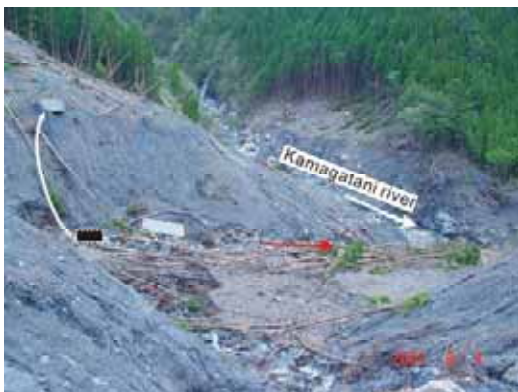
Photo 11 A displaced concrete block from the soil-conservation (check) dam (Black area outlined by the broken white line) on the slope opposite the landslide source (Red arrow: downstream of the valley; White curved arrow: move direction of the block)
