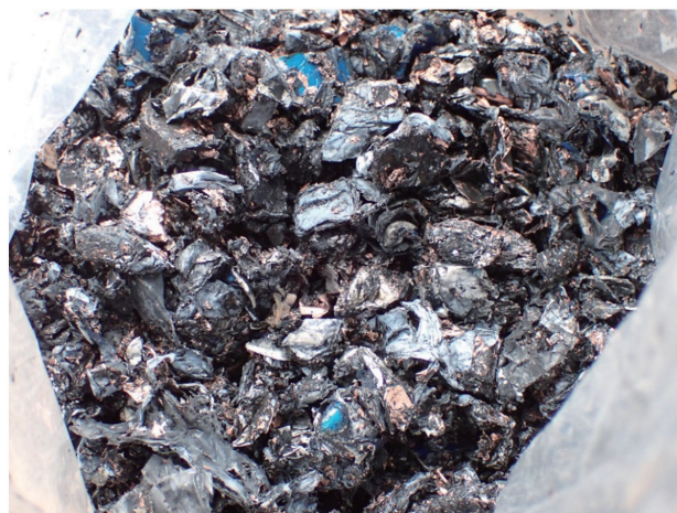
Fig. 4 A photograph of the sample obtained by the submerged crushing of the prismatic LIB cells dismantled from a hybrid electric vehicle in lime water under N 2 flow.
