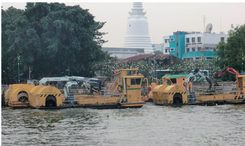
Floating machines to remove water Hyacinths, Bangkok
